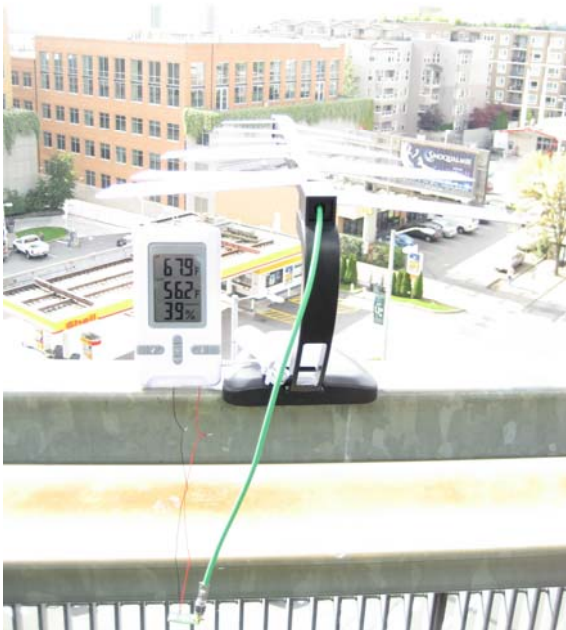
Fig. 7. Operating a temperature and humidity meter (including LCD display) using only ambient RF power.
